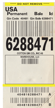
PBI tag: The first two digits of the gin code identify the classing office, followed by three digits identifying the gin. The remaining seven digits identify the bale.
