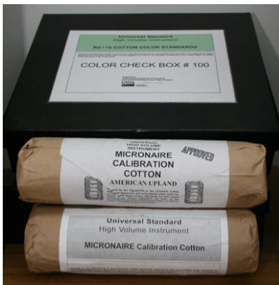
Examples of Universal Color Standards and Micronaire Standards for high volume instrument calibration.
