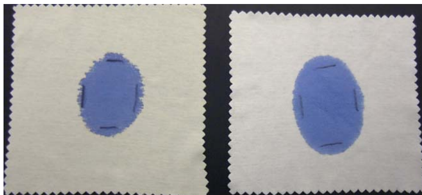
Figure 3. Horizontal spread of a cotton fabric with minimal scour (left) and improved scour (right).
