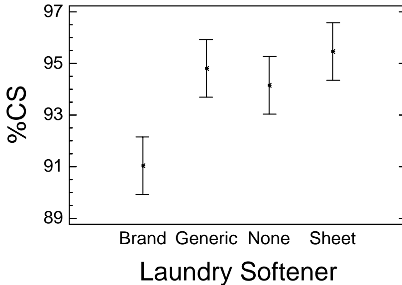
Figure 4. Mean %CS and 95% confidence limits for various types of home laundry softeners.
