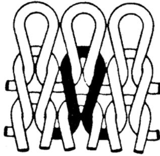
Figure 1 - Ideal alignment of course and wale loops. Wale loops are vertical and course loops are horizontal.
