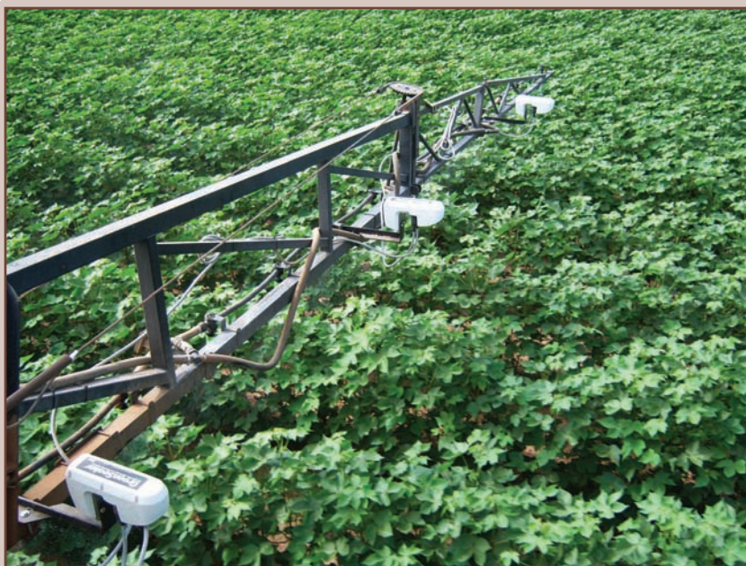
Figure 4. Example sensor-based system using GreenSeeker sensors mounted along the sprayer boom.
