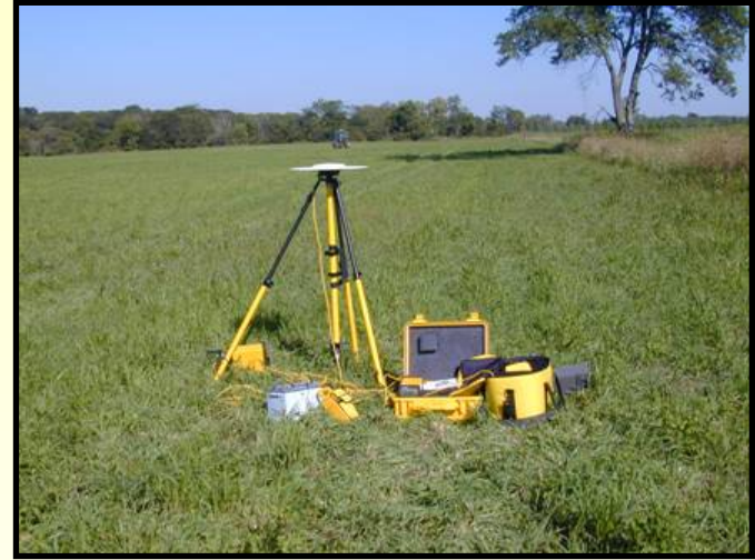
RTK Base Station with radio
