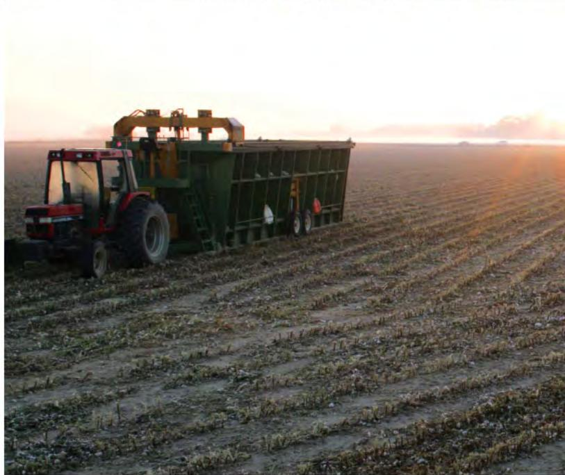
**NOW** New machines from Case IH and John Deere both pick the cotton and form the modules on the harvester.
