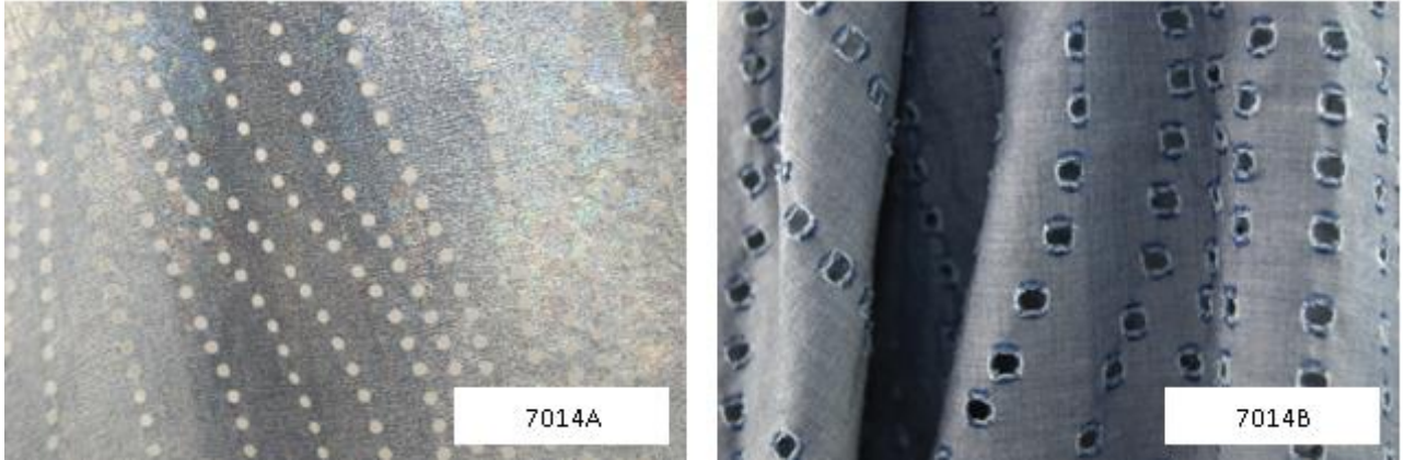
Figure 10. Foil adhesive seals cut edges and prevents fraying
