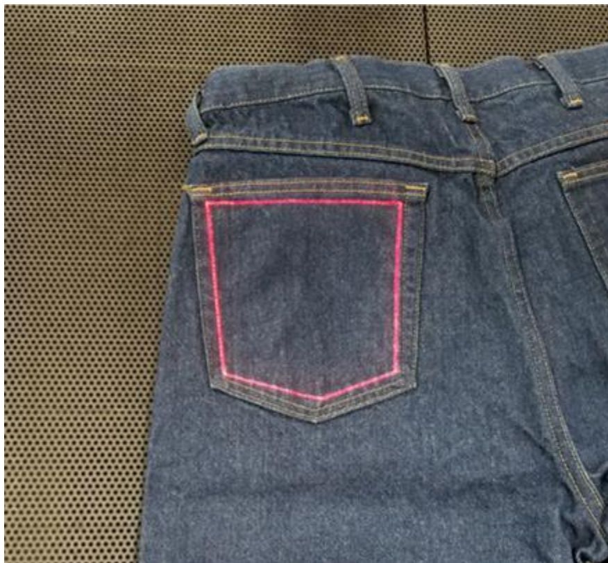
Figure 2. Visible red laser outline for positioning garments.
