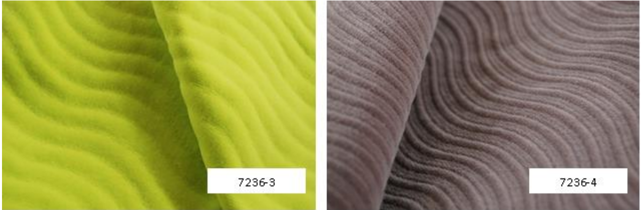
Figure 12. Demonstration of the results achieved by varying the marking speed of lines in laser vector files
