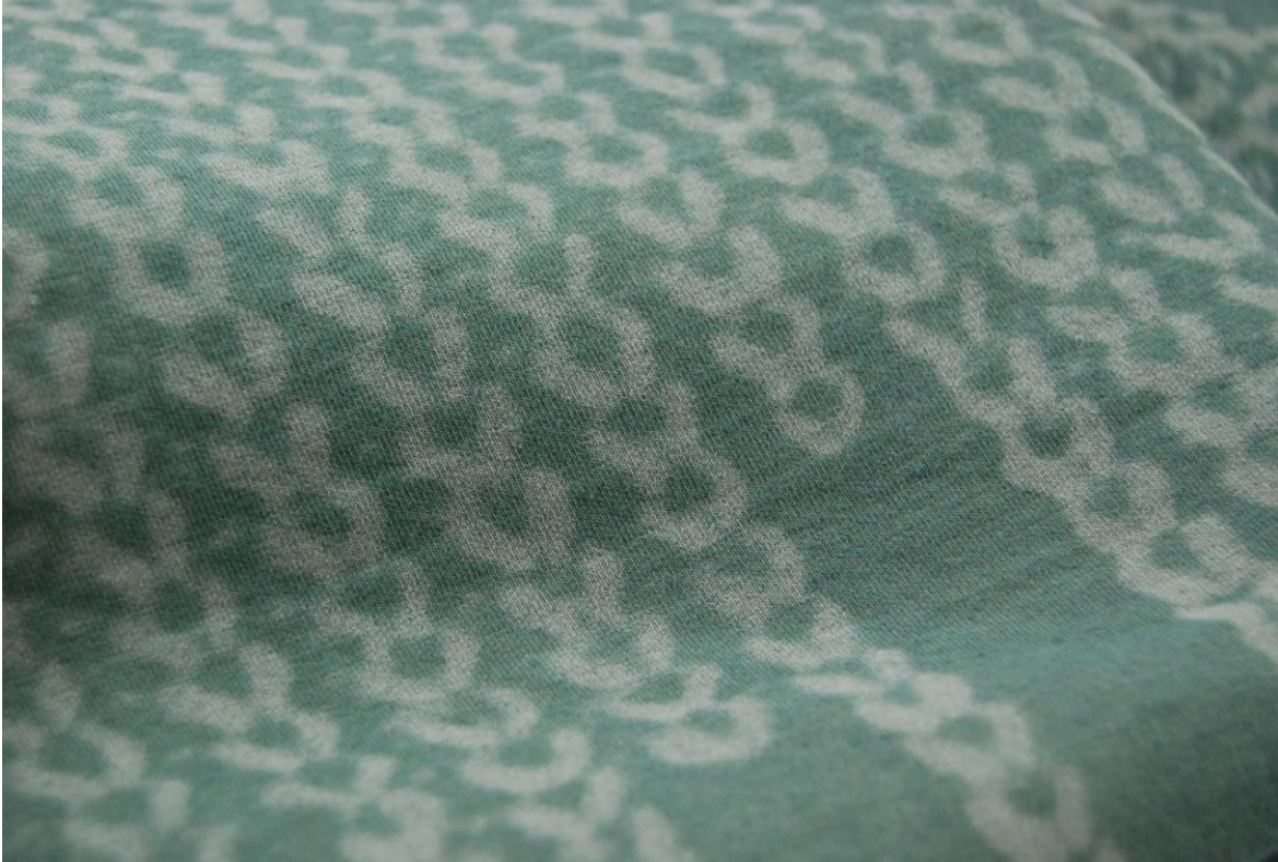
Figure 9. FABRICAST DK-2747-1L Marking an image with a laser on reactive dyed spacer knit.
