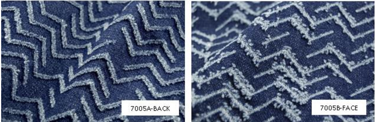
Figure 11. Demonstration of the results achieved by scoring the back vs. the face of a fabric using a laser vector file
