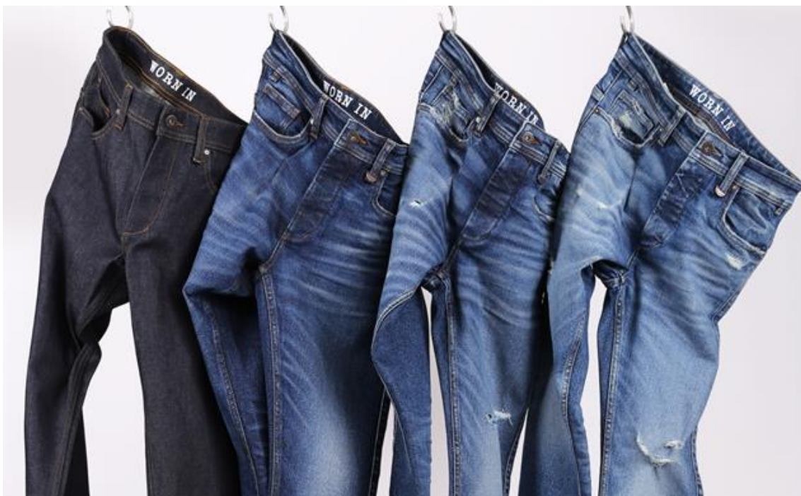
Figure 1. A series of sample garments produced by Soorty denim mills to demonstrate laser finishing techniques from unprocessed (left) to heavily altered (right).
