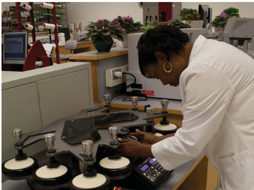
Tara Smith, Laboratory Assistant in the PEL at Cotton Incorporated, conducts abrasion resistance tests on multiple specimens simultaneously on the new Martindale tester.
