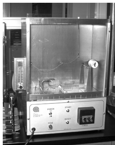
Flammability test apparatus for general wearing apparel fabrics.
