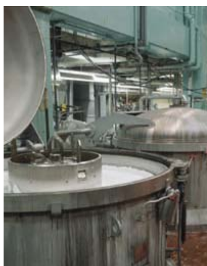
Patented Kier bleaching system.
