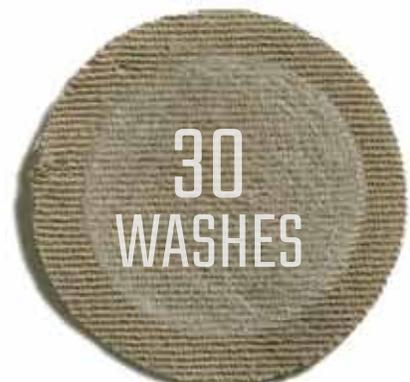
ASTM D4966 - MARTINDALE TRIZACT ABRASION TEST - 300 CYCLES, TWILL FABRIC
