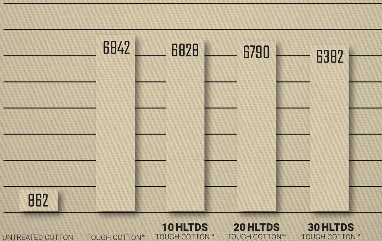
ASTM D3885 - # OF CYCLES TO BREAK, TWILL FABRIC
